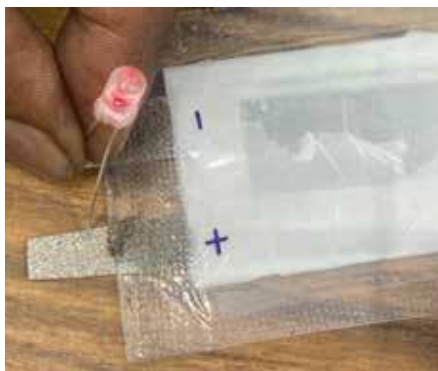
Figure 1. Zn-Ni-Co oxide//AC/rGO asymmetric supercapacitor device
