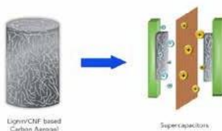
Figure 1. Schematic diagram for energy storage devices using Lignin/CNF based carbon aerogels
